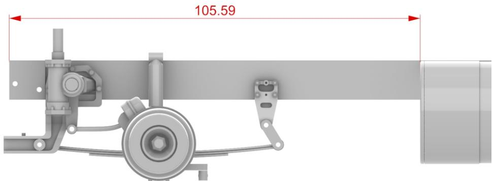
8. Distance between front end of frame and front end of battery box.
