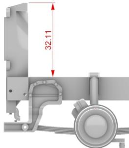
6. Distance between front end of frame and rear cab's supports.
