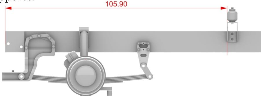
7. Distance between front end of frame and front end of fuel tanks.
