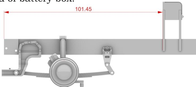
9. Distance between front end of frame and silencer's brackets.
